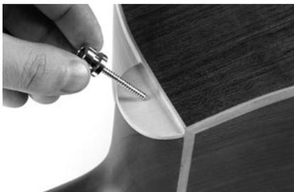
Install the strap lock only at the neck point, which is strong enough to hold the screw. Drill a hole with a 2mm wood drill first.
