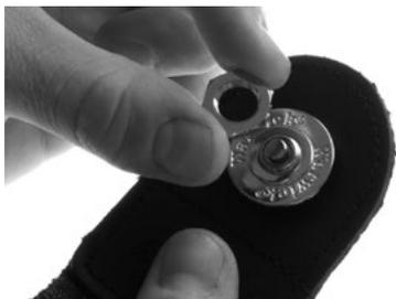
Screw the nut on the thread. Tighten with a wrench.
