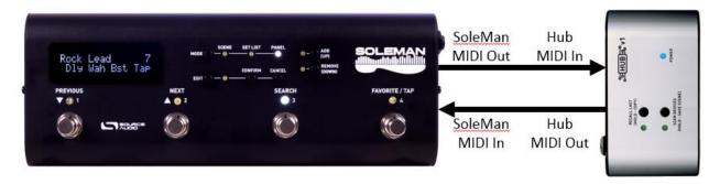
After the MIDI cable connections have been made, navigate to the "Use Hub Names" screen in the Edit Menu and use the Previous/Next footswitches to set the value to "Yes."
