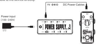
If the input polarity of the electrical device is , please connect polarity reversal cable to the DC power cable, then connect the device
