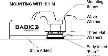
Note: Mounting procedures apply to all three mounting screws.
