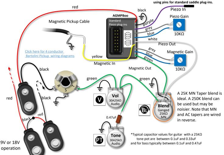
This Sample wiring diagram is not meant to represent what is included with the AGMPBoo but is only a suggestion of how it may be used in an instrument with 1 magnetic pickup and piezo pickup(s). See the product page for details. <u>https://bartolini.net/product/agmpb/</u>
