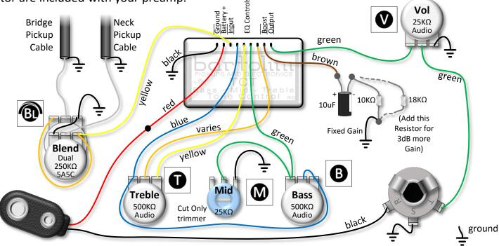
The negative side of the battery should be connected to the jack ring so that power is turned on only when the plug is in. Unplug the instrument when not in use to conserve your battery. Ensure bridge and cavity shields are connected to ground.
