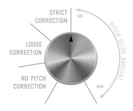
Hedra features 3 different pitch corrections settings or a pitch glide amount as listed in the knob graphic below. When Loose Correction is selected, the notes are forced into the current Key and Scale but pitch bending is not removed from the input. When Strict Correction is selected, the notes are forced into the current Key and Scale but pitch bending is removed from the input.
