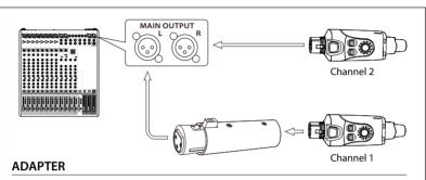
If the XLR inputs/outputs on your mixer are very close to each other, using the XLR adapter with a transmitter/receiver allows you to plug in two transmitters/receivers side-by-side.
