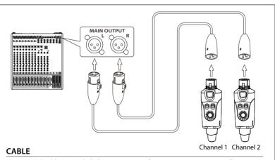
Using an XLR cable (not included) as an extension for a transmitter or receiver allows you to connect the components to a mixer where the inputs/outputs are very close together. It can also resolve wireless signal interference issues if you have too many wireless units in close proximity to each other.
