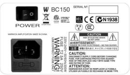
For your safety, remember to plug the power cord into the amplifier first and then into the wall outlet before turning on the POWER switch.
