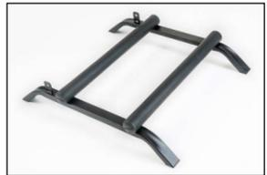
2. Take the **risers (3)** and screw them to the angled flaps on the **feet (2)**. Use a **short socket screw (D)**, a **washer (E)** and a **cap nut (H)** to fix the **risers (3)** to the **feet (2)**. Use the **wrench (A)** and **hex key wrench (B)** to tighten the nuts.
