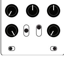
Use an expression pedal to morph from forward (heel down) to reverse (toe down). Set **SPEED** to 12:00 for tape stop effect.
