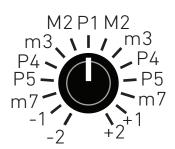
**PITCH**: -2 to +2 octaves—Pitch shifting. No pitch shift in middle position (12:00). In live play mode, pitch shifting happens in realtime. In hold modes, the loop playback speed is changed to maintain the best fidelity. You can combine the **PITCH** and **TIME** controls to adjust the pitch and loop length independently. The **PITCH** knob is quantized to intervals.
