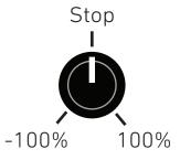
SPEED: -100% to +100%—Tape speed effect. Smoothly changes the playback speed, from forward (clockwise) to reverse (counter clockwise). In the middle, the sound is stopped. Reverse playback will play short segments of audio backwards, simulating studio tricks where a tape is flipped over to create a reverse guitar solo. The Tensor analyzes your playing to automatically adjust the size and timing of the reversed segments (See NXT hold mode or "Drift" if you need more control).
