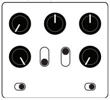
Using **NXT** mode gives you more control over the timing of reverse playback. Tap **HOLD** twice to set the length of each reversed slice.
