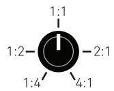
**TIME**: 1:4 to 4:1—Time stretch/compression. Normal playback is in the middle position (12:00). To the left, playback is stretched without pitch shifting. To the right, playback is compressed without pitch shifting. Time compression only works during loop playback; during live play and recording it will play at normal speed (since it cannot hear the future). Stretching or compressing more than 2x will introduce glitches, which you can use to create new textures.
