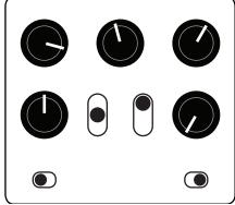
PITCH shift up slightly, then use SPEED to bring pitch down until it is slightly detuned. TIME stretch slightly to separate voices. RAND at 8:30 will add occasional instability.
