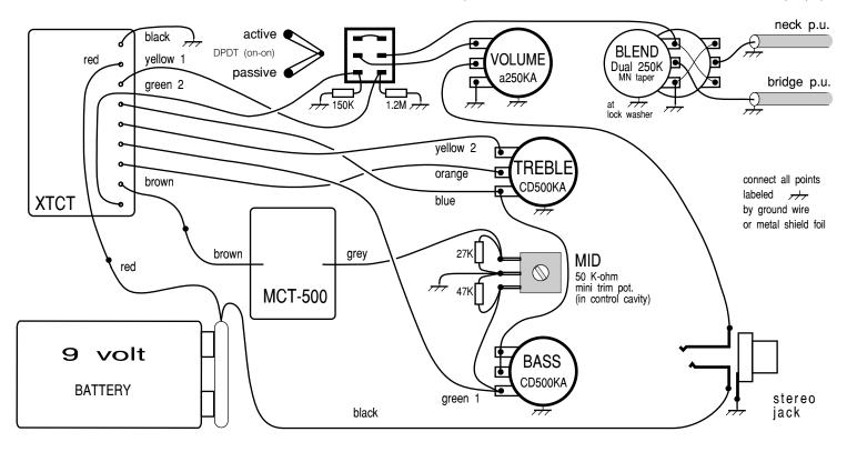
XTCT in 2 pickup instrument with 2 Volumes and Treble/Bass (Dual Concentric)
