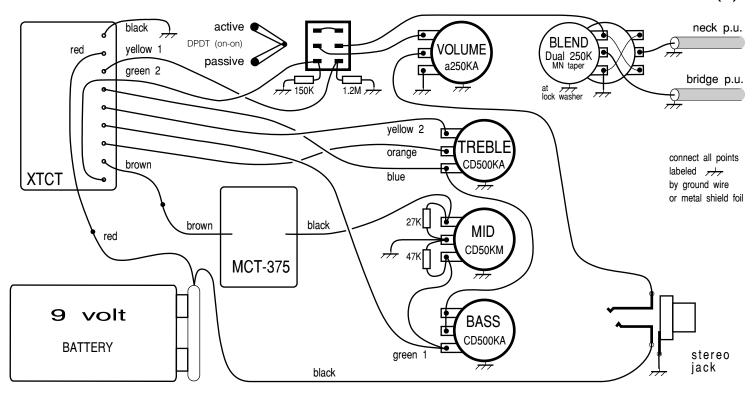
XTCT in 2 pickup instrument with Volume, Blend, Treble/Bass (Dual Concentric) and Mid Controls with Active/Passive Switch and Mid Boost Module (6)
