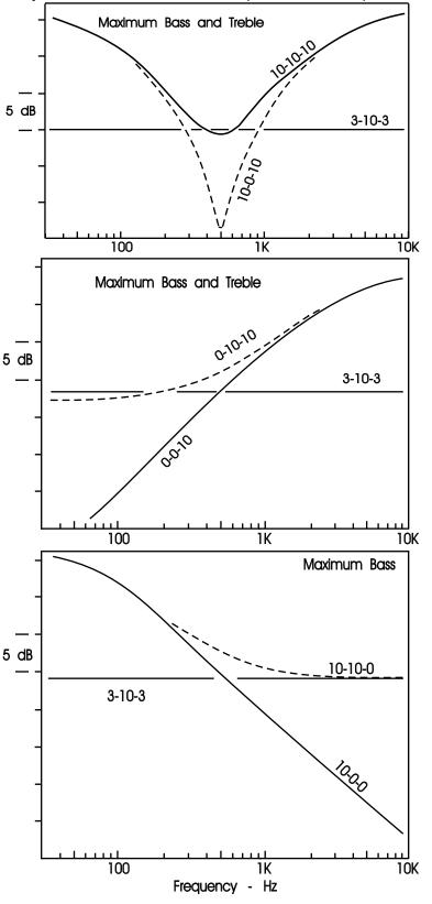
XTCT in 2 pickup instrument with Volume, Blend, Treble, Mid & Bass Controls with Mid Boost Module (1)
