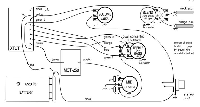
XTCT in 2 pickup instrument with Volume, Blend, Treble and Bass Controls with Active/Passive Switch & Mid Boost Module (Mid Boost/Cut by mini trim pot.) (3)
