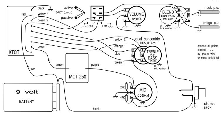
XTCT-LZ with DTA 1.3 buffer with Volume, Blend, Treble, Mid & Bass Controls with Mid Boost Module (7)
