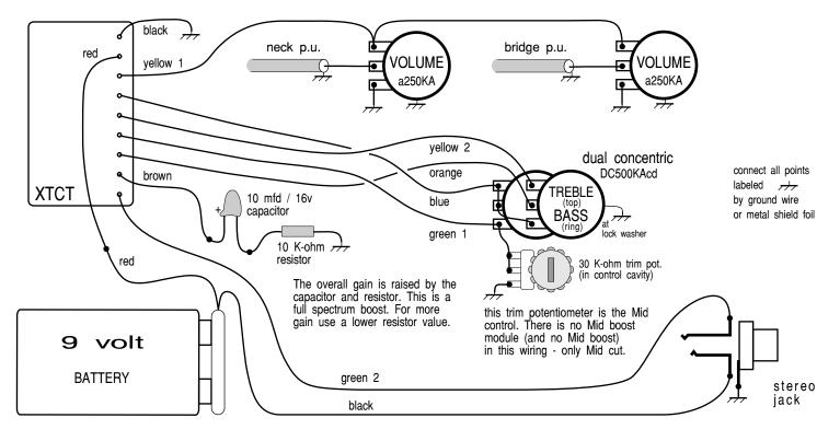
XTCT in 2 pickup instrument with Volume, Blend, Treble, Mid and Bass Controls with Active/Passive Switch and Mid Boost Module (5)
