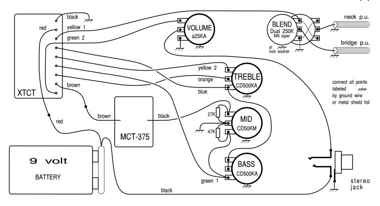
XTCT in 2 pickup instrument with Volume, Blend, Treble/Bass (Dual Concentric) and Mid Controls with Mid Boost Module (2)
