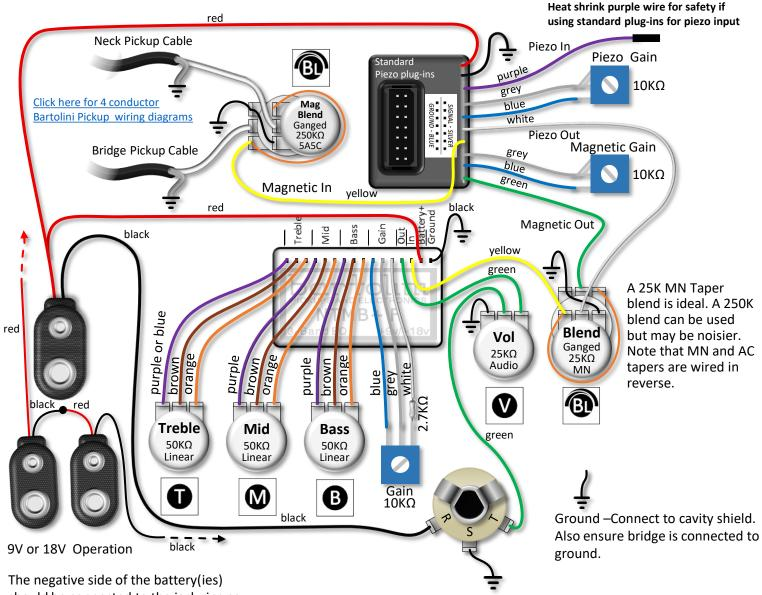
The negative side of the battery(ies) should be connected to the jack ring so that power is turned on only when the plug is in. Unplug the instrument when not in use to conserve your battery.
