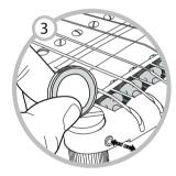
Adjust the two set screws at the back of the bridge so that the range of travel of the saddles is beyond the scale length measured from the nut (scale length is 2x the distance from the nut to the 12th fret).
