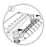
Remove the strings and remove the old bridge by sliding it off the posts. The ResoMax bridge comes with steel posts that enable the magnetic AutoLock feature. You may keep using your old posts if they are also steel.
