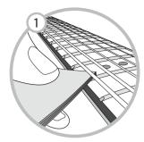
Determine correct string height by measuring the gap between the top of the 12th fret and the bottom of the low E string. It should be around 0.125" (3mm), or about a stack of a 12 cards if you don't have a ruler. For the high E string, the gap should be around 0.080" (2mm) or about a stack of 8 business cards.
