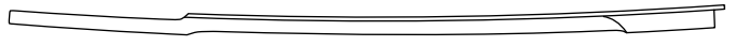
Loose truss rod with up-bow in the neck (concave), high string action.
