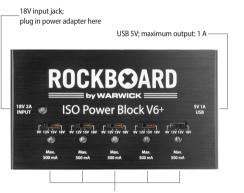
5 x switchable slots with 9V DC / 12V DC / 15V DC / 18V DC; Individual maximum output: 500 mA at 9V, 375 mA at 12V, 300 mA at 15V, 250 mA at 18V
