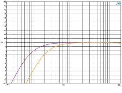
High-Pass filter response -3dB corner at 80Hz or 200Hz
