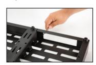
Once the tips of the screws are sticking out on the other side of the holes and the screws become easier to turn, the threads have been cut properly. Now remove the screws again.
