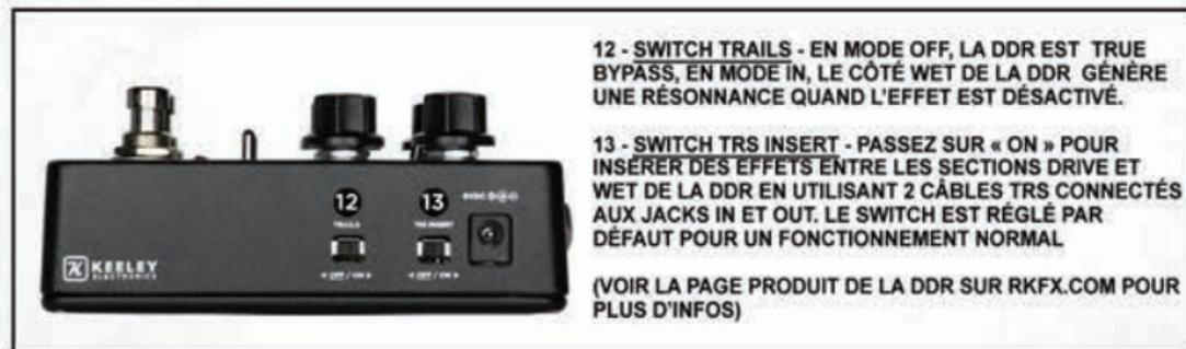
12 - SWITCH TRAILS - EN MODE OFF, LA DDR EST TRUE BYPASS, EN MODE IN, LE CÔTÉ WET DE LA DDR GÉNÈRE UNE RÉSONNANCE QUAND L'EFFET EST DÉSACTIVÉ.
