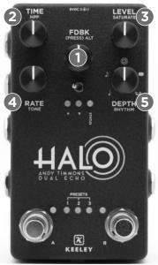
Hold down the FDBK knob while manipulating other knobs to access secondary controls.
