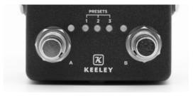
**SIDE A / B** - Tap the A or B footswitch to activate each side of the HALO. Tap the alternate footswitch to use the alternate sound stored in each Preset Bank.
