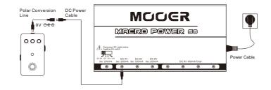
If the input power of the electrical device is not 9V, please use the adjustable voltage output jack and its voltage switch to match the same output power of the electrical device before plugging it to the MACRO POWER.
