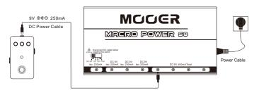
If the input polarity of the electrical device is ⊕⊕⊕, connect a polar conversion line to the DC power cable before connecting the device.
