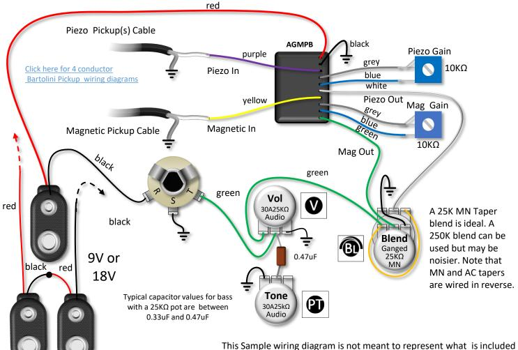
The negative side of the battery(ies) should be connected to the jack ring so that power is turned on only when the plug is in. Unplug the instrument when not in use to conserve your battery.
