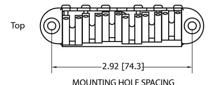
NOTE: For use on new guitar builds. Cannot be used for existing guitars as a bridge upgrade
