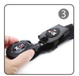
Put the U2 Transmitter into the holder.
