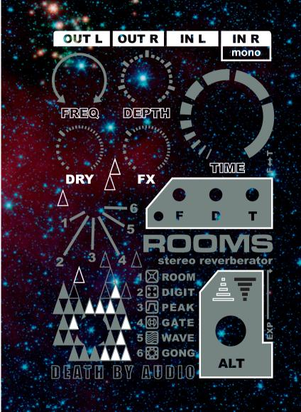
**CONNECTIONS:** Plugging only in to **IN R** mono splits the dry uneffected signal to both outputs. Plugging in to **IN L** separates the L and R clean signals to their own outputs. The effected signal always cascades for an expanded stereo image.
