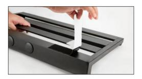
**STEP 3**Apply self-adhesive loop tape or another reusable fastener to the position on top or underneath your pedalboard where you want to place your MOD 4.
