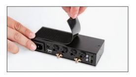
Apply self-adhesive hook tape or another reusable fastener to the bottom of the MOD 4 housing.
