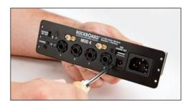
**STEP 1**Detach the MOD's front plate by removing the marked screws.
