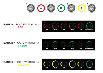
The colour of the CHANNEL CONTROL LED's will indicate which BANK is currently selected. After selecting a different bank the PREAMP LIVE will wait for you to select a channel within that bank before changing the sound.
