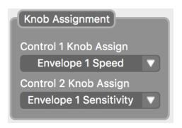
Use the Control 1 Knob Assign and Control 2 Knob Assign dropdown menus to select which parameter are assigned to CONTROL 1 & CONTROL 2 knobs on the face of the pedal.
