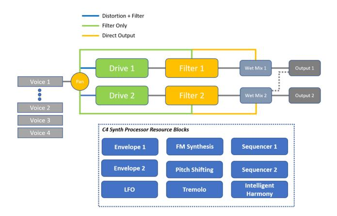
**Step 1. The Voices**: First in line are the C4's Voices (there are four of them, hence the name "C4"). Assigned each activated Voice to its own Sound Source (Sine, Square, or Saw Oscillator / Monophonic Pitch / Polyphonic Pitch / Dry Signal). Mix together multiple Voices to create a single amazing preset.
