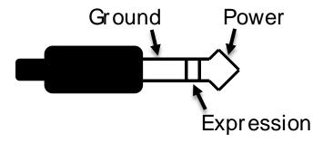
Expression pedals with TS (Tip Sleeve) plugs will not work correctly with the C4.
