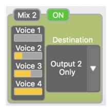
Mix 1 and Mix 2 Blocks: The four meters labeled Voice 1 through 4 monitor the signal ratio routed through Processors 1 & 2. Please note that setting the Destination of Mix 1 to Output 1 Only and Mix 2 to Output 2 Only is necessary in creating stereo effects. Each Voice's position in the stereo spread is set with the Processor Pan control in each of the Voice blocks.
