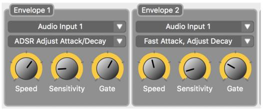
The Envelopes control amplitude and filter modulation of the each C4 Voice. Both Envelopes 1 and 2 run independently of each other and each can be assigned a different set of Voices.
