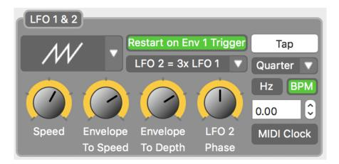
The LFOs (Low Frequency Oscillators) can be set to control the Filter modulation, Sequencer rates, or Tremolo rates (amplitude modulation).
