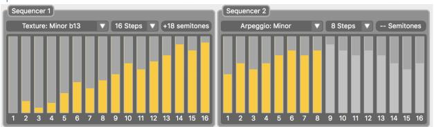
The C4 features two simultaneously running Sequencers. With the Sequencers it is possible to create two note patterns up to 16 steps long. The Sequencers come with 16 different pre-made sequences all of which can be edited into your own custom pattern. Please note that Sequencer 1 responds to Voices assigned to a Source labeled with a "1" (ex. Square 1, Sine 1, Saw 1) and Sequencer 2 responds to Voices assigned to a Source labeled with a "2" (ex. Square 2, Sine 2, Saw 2).
