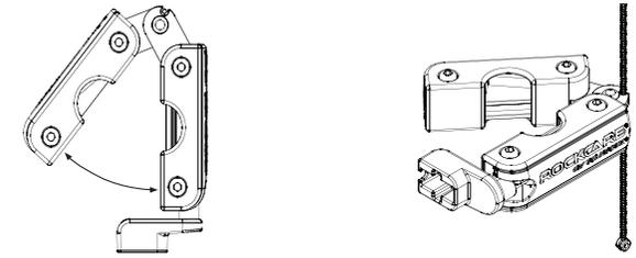
Your MultiTool comes with exchangeable string winders for guitar and bass. These can be easily exchanged by pulling them off the axis of rotation. The guitar version has an additional bridge pin puller.
