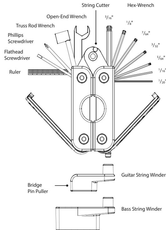
All the different tools are safely contained in the two halves of the housing.
