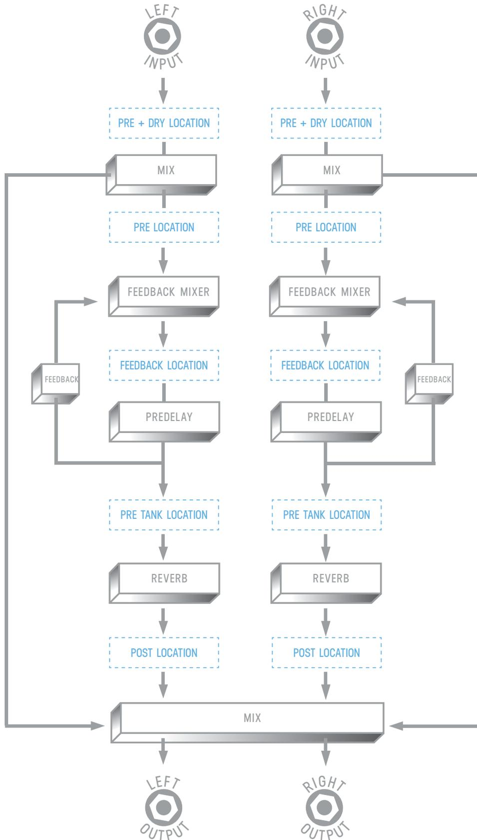
Also shown in the visual diagram is the Mixer for MercuryX. The Mixer is directly connected to the front panel mix knob. To adjust the Dry and Wet Trim levels, use **C3** to enter Edit View and page over to the MIX section. The following is a breakdown of each Category and the processing Elements they contain:
