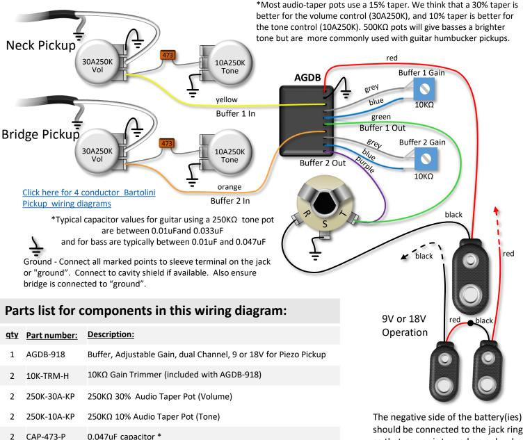
should be connected to the jack ring so that power is turned on only when the plug is in. Unplug the instrument when not in use to conserve your battery.
