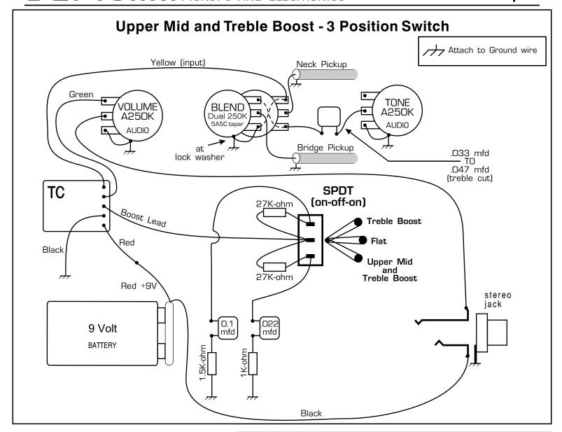
The 0.1 mfd and 0.022 mfd Capacitors control the frequency of the boost. Larger capacitors boost more of the bass frequencies. A 10 mfd capacitor will boost all frequencies equally (flat boost). The 1.5K-ohm and 1.0K-ohm resistors limit the amount of boost, larger resistor values decrease he boost levels.
