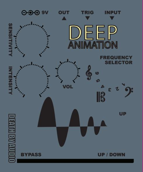
**INPUT** Plug an instrument into this jack.
