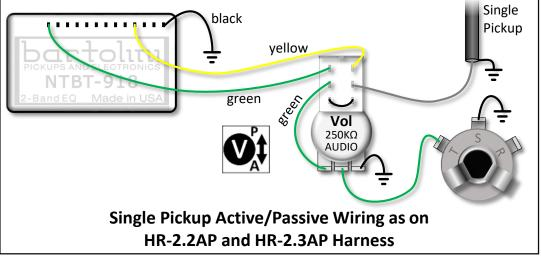
Ground – Connected to preinstalled bare wire.
