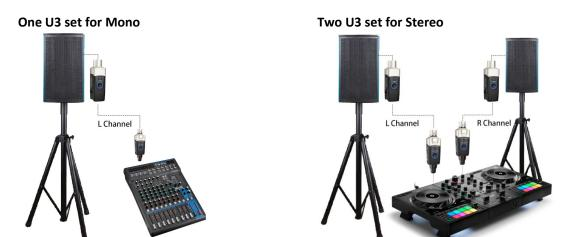
One U3 transmitter can transmit to multiple receivers, so you can send the same signal to several speaker cabinets simultaneously! This allows you to send a mono signal to two or three or four (or more) powered cabinets/monitors; or, with a stereo setup, a separate U3 system can be added on a different wireless channel, with multiple receivers connected to multiple powered cabinets. This allows you to fill any venue with sound!
