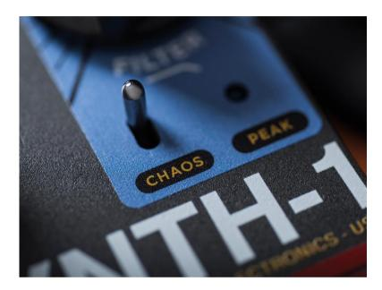
The Chaos toggle introduces glitchy tones by making note tracking less stable
