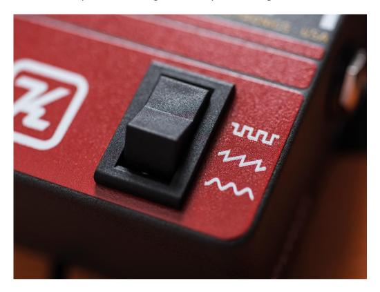
Select between square, sawtooth and sine waveforms to change the basic character of your guitar tone, then adjust further with the filter controls
