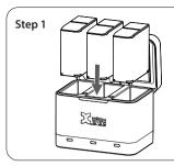
Insert the U5B batteries into the charger so that the battery and charger connectors line up.
