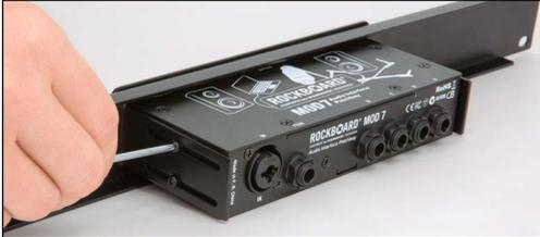
Place your **RockBoard®** MOD in the mounting slot and use the included TX10 screwdriver to screw the M3 x 4 mm screws through the assembly bracket into the threads on both sides of your MOD to lock it in position.
