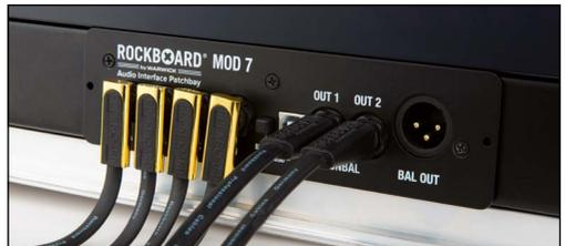
When the **RockBoard®** 19" Rack Panel is safely mounted, you can connect your cables and start to use the MOD.
