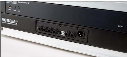
The detachable front plate of the **RockBoard®** MOD unit is higher than 1 U, so it might overlap your rack units above or below the **RockBoard®** 19" Rack Panel. If this causes problems, you can remove the front plate from your MOD by removing the screws using a PH2 Phillips head screwdriver. The mounting nuts of the jack sockets do not need to be removed.
