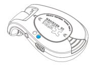
The LED on the receiver will stop blinking after the connection was successfully established.
