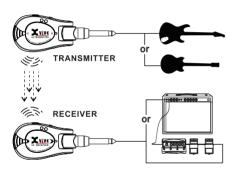
Transmitter plugs into your guitar (or other instrument), the receiver plugs into the effects pedal, amp or other audio device.
