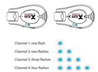
Turn transmitter and receiver on and verify that the blue LED flash the same number of times on both devices to indicate that they are operating on the same channel.
