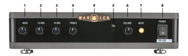
**Tone Stack**: The active 4-band EQ section provides up to +/- 15 dB of cut or boost for each band. Controls set to the center position (detent at 12 o'clock) provide a flat / neutral response for that band. Turning the knobs clockwise boosts the frequency band, while turning the knobs counterclockwise cuts the band.
