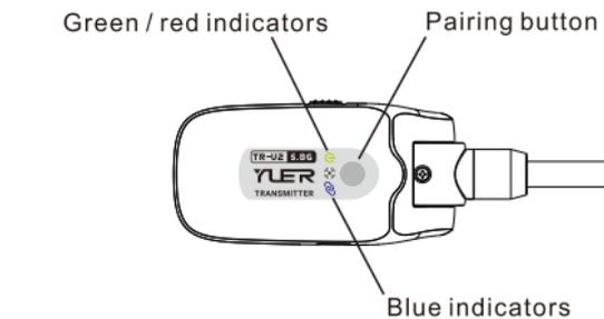
Switch on the transmitter and receiver, press and hold the pairing button for more than 2 seconds until the blue indicators are flashing blinks. Then wait for the auto pairing. When the blue indicators of both transmitter and receiver are always on, it means the pairing is successfully.
