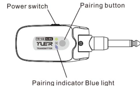
Switch on the transmitter and receiver, press and hold the pairing button for more than 2 seconds until the blue indicators are flashing blinks. Then wait for the auto pairing. When the blue indicators of both transmitter and receiver are always on, it means the pairing is successfully.
