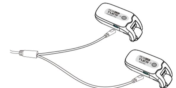
★ The double-sided USB cable can charge the transmitter and receiver simultaneously.
