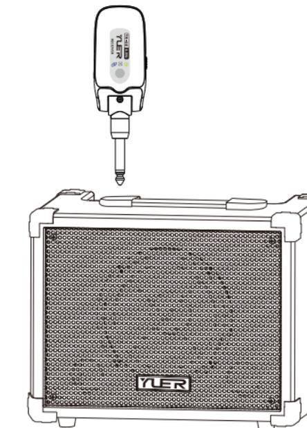
Switch on the receiver, if its blue indicator is on, it indicates the receiver and transmitter are paired . If the blue indicator is flickering , it indicates they're not paired, it might due to strong signal interference, exceeds transmission distance or Need to pair again.
