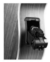
The battery and electronics compartment can be easily opened with your fingernail. Push the battery in until it locks in place.
