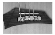
Place the string's ball end on the bridge string holder. Hold the ball end down with one hand and with the other feed the string to the tuner.
