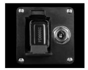
The battery compartment is located directly beside the output jack. You can easily open the compartment with your fingernail. Push the battery in and close the lid. Please mind the correct polarity!
