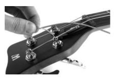
The tuner's post has a slot with a hole in the center. Put the string in that hole before you start winding. This system avoids the string poking out to the side of the tuner and stabilizes the winding and thus the tuning overall.
